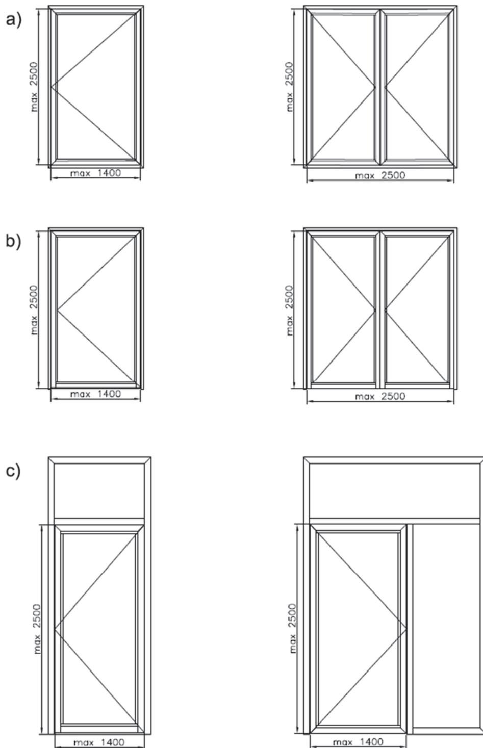
**Fig. 6 Types of fire constructions rated EI90 and leaf maximum dimensions:
