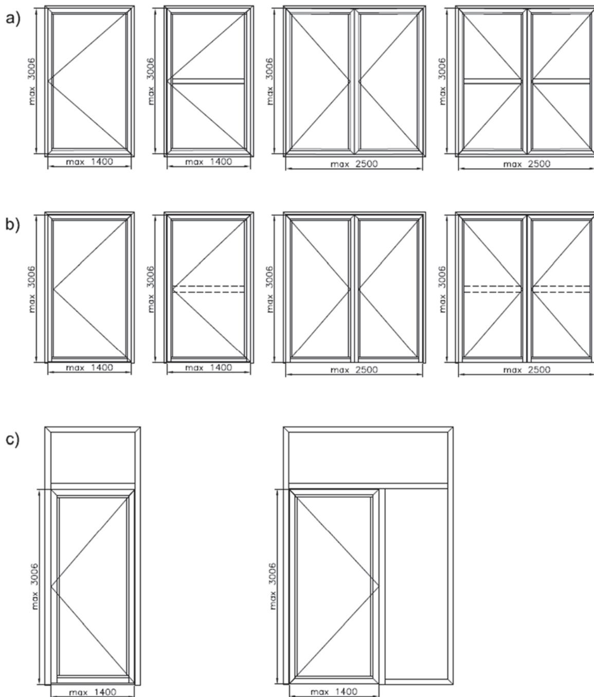
**Fig. 4 Types of fire constructions rated EI30 and leaf maximum dimensions:
