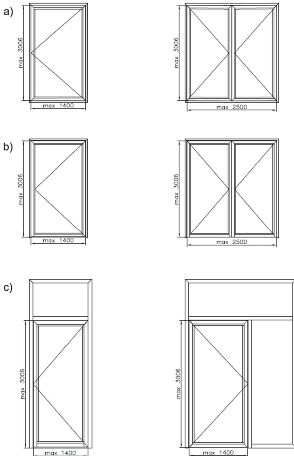
**Fig. 5 Types of fire constructions rated EI60 and leaf maximum dimensions:
