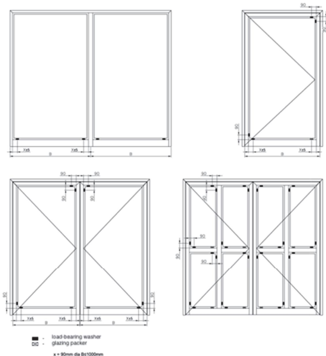
**Fig. 46 'Push-out' of glazing in door leaf/frames. Rules for placement of glazing packers,  $x = 90\text{mm}$  for  $B \leq 1000\text{mm}$**
