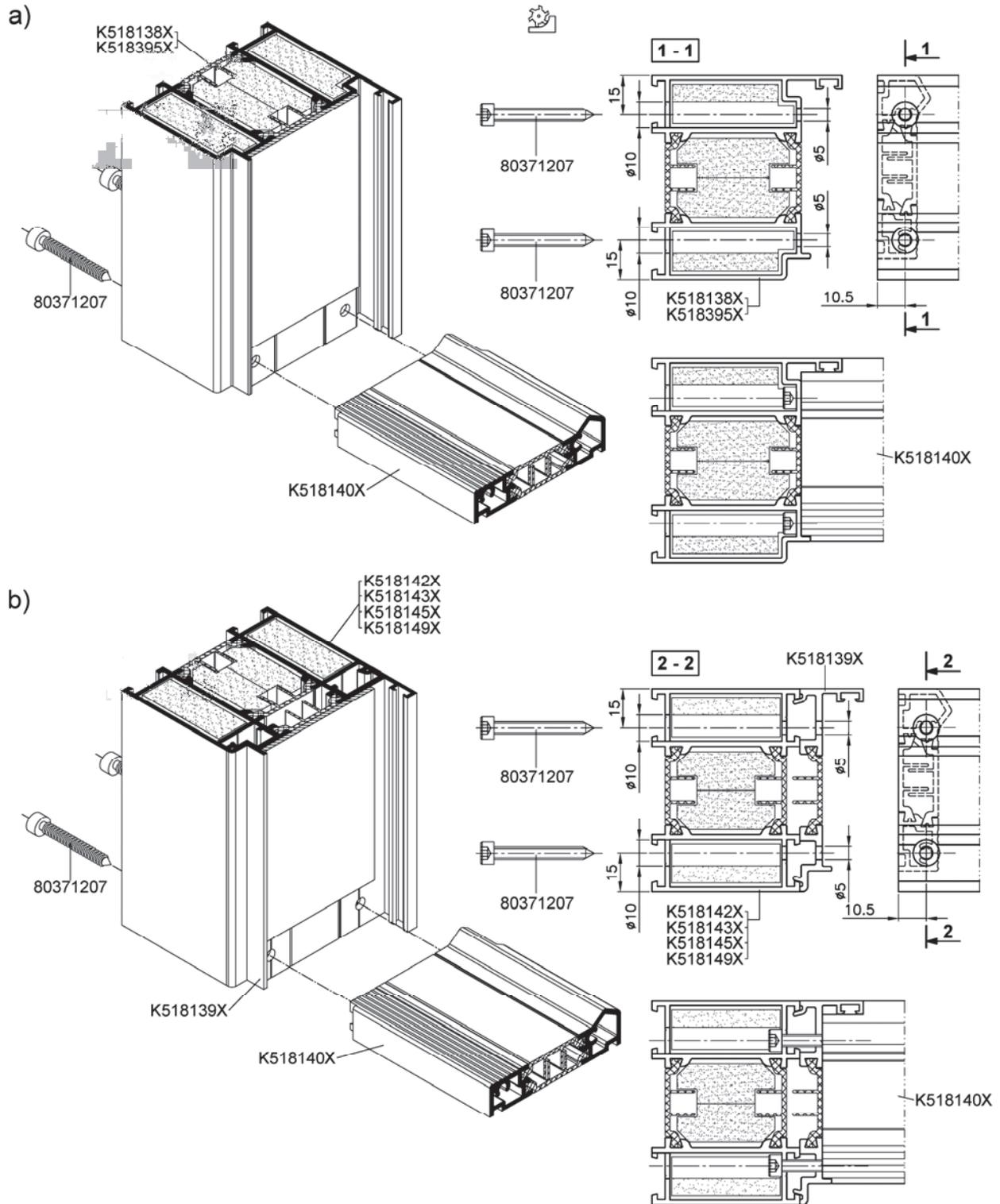
**Fig. 32 Threshold installation for EI 30 and EI 60 doors:**
