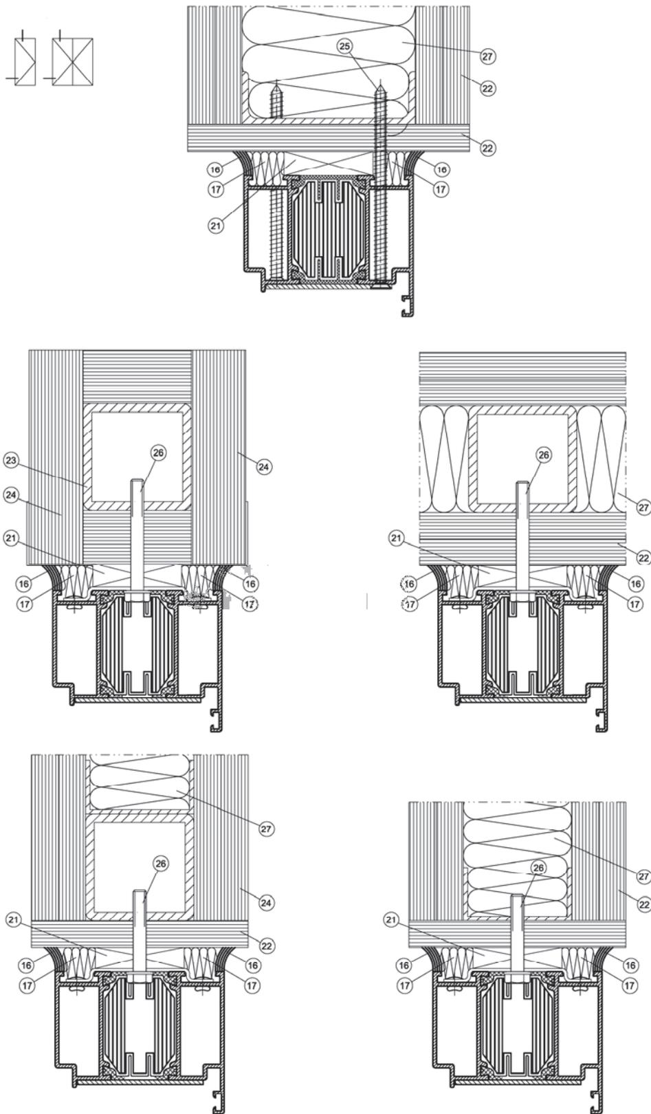
**Fig. 21 Sealing variants for frame connections in doors, technical windows and door system frames rated EI30, embedded in framed flexible walls clad with plasterboards**
