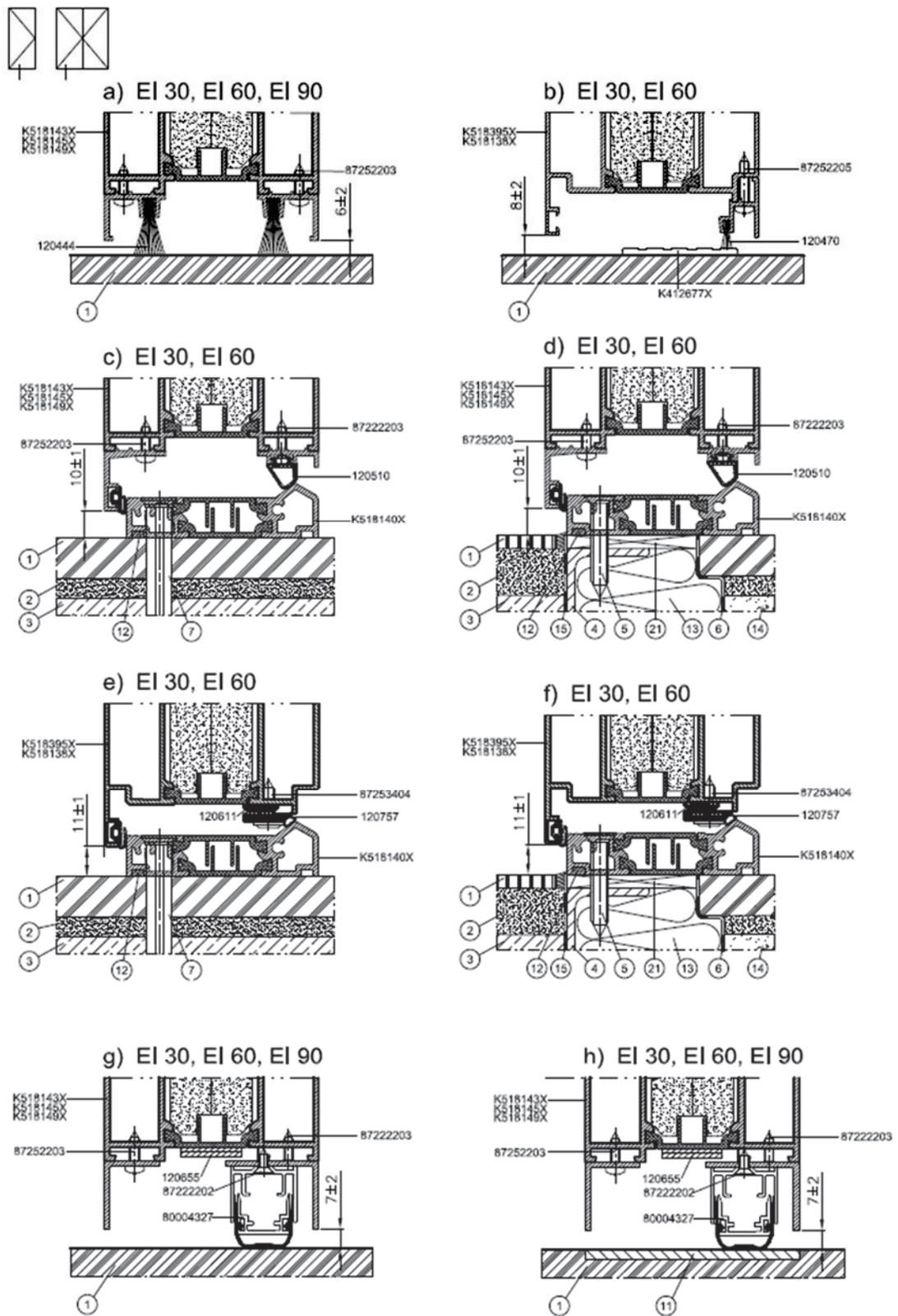
Fig. 27 Variants of door stop sealing – clearance between floor and leaf
