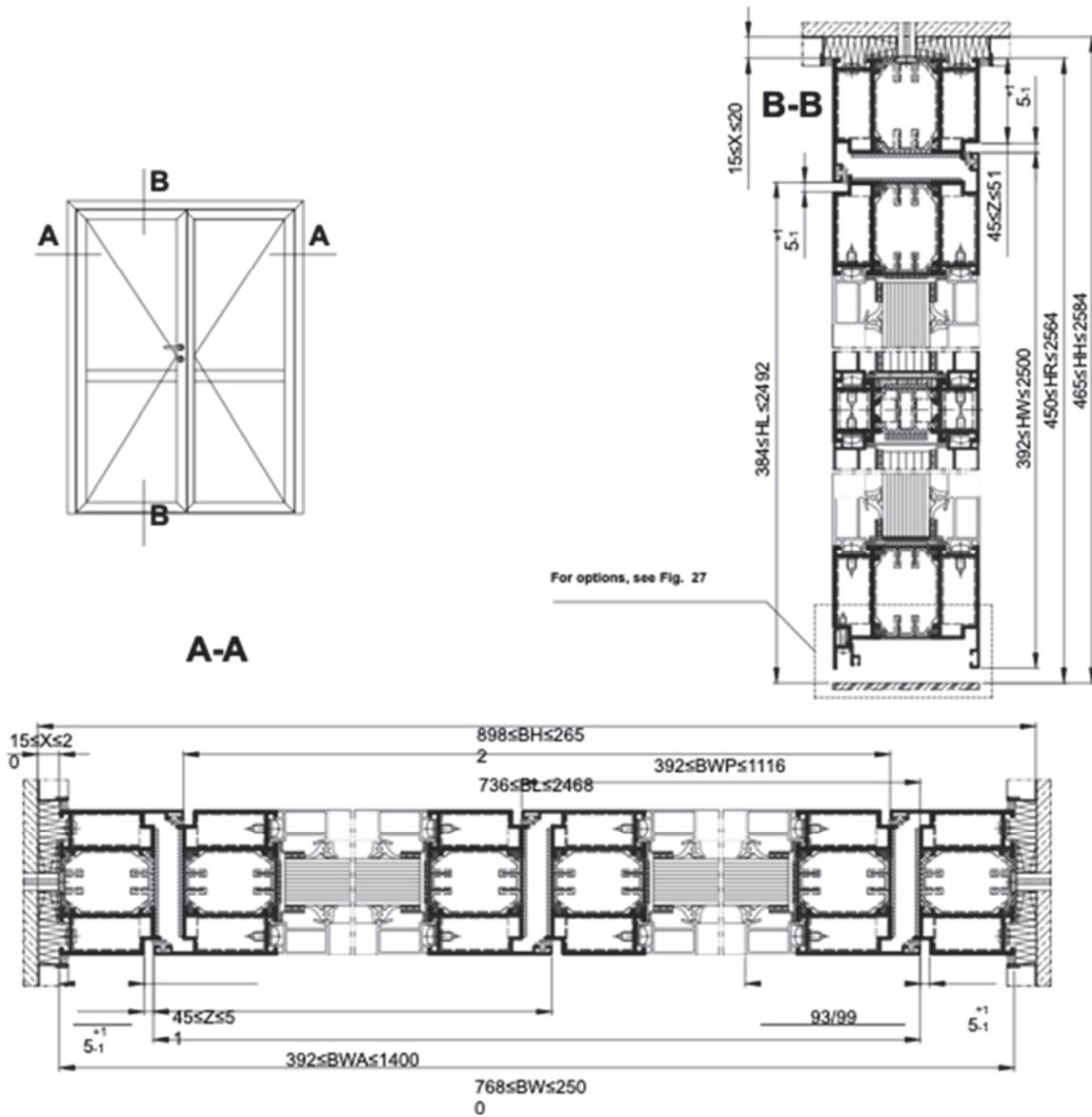
Fig. 15 Dimensional specification of the installation of single door MB-78 EI90
