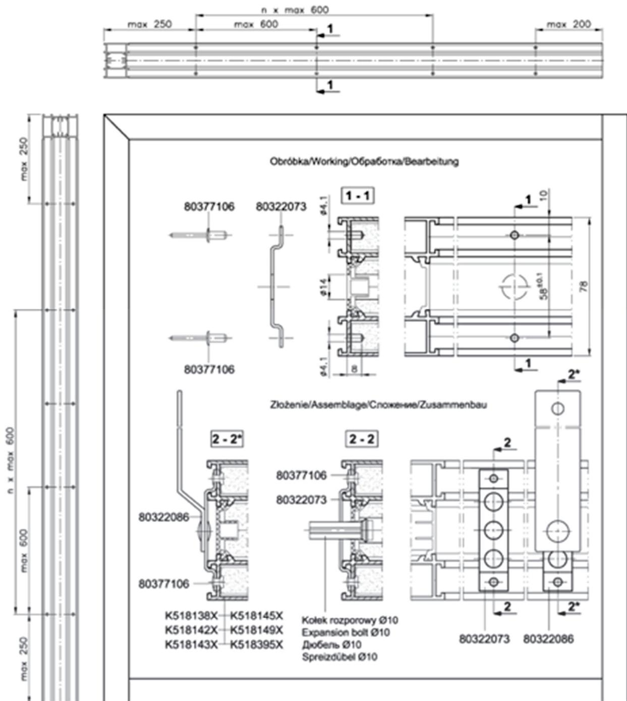
Thru-drill a  $\varnothing 14$  hole when fixing with expansion bolts. Drill a  $\varnothing 4.1$  hole using the device P3K-837-03.
