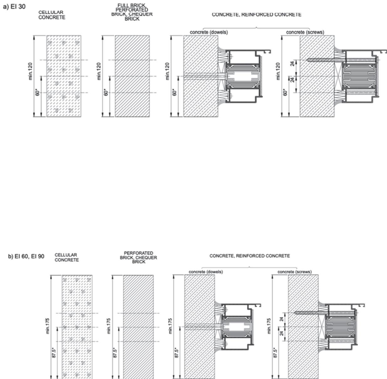
Fig.3. Recommended distance of dowels and screws from the edge of the frame for walls made of various building materials (required wall density: min. 650kg/m<sup>3</sup>)
