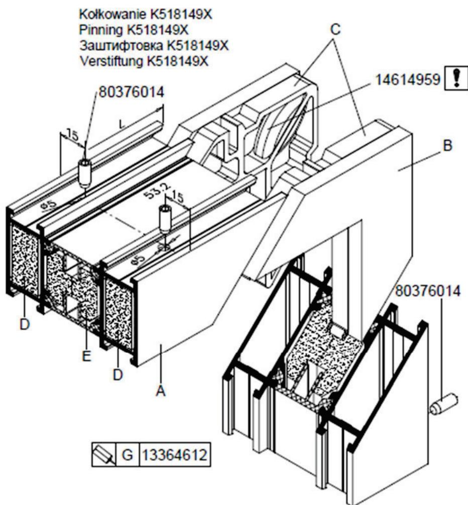
Fig. 22 'L' connections for circumferential door system frames
