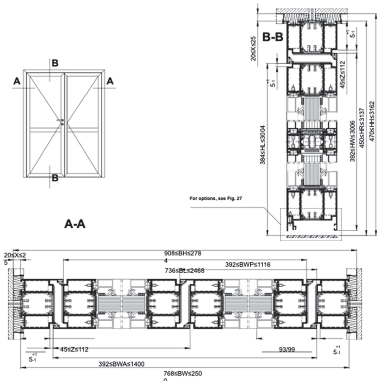
Fig. 14 Dimensional specification of the installation of single door MB-78 EI30 and MB-78 EI60
