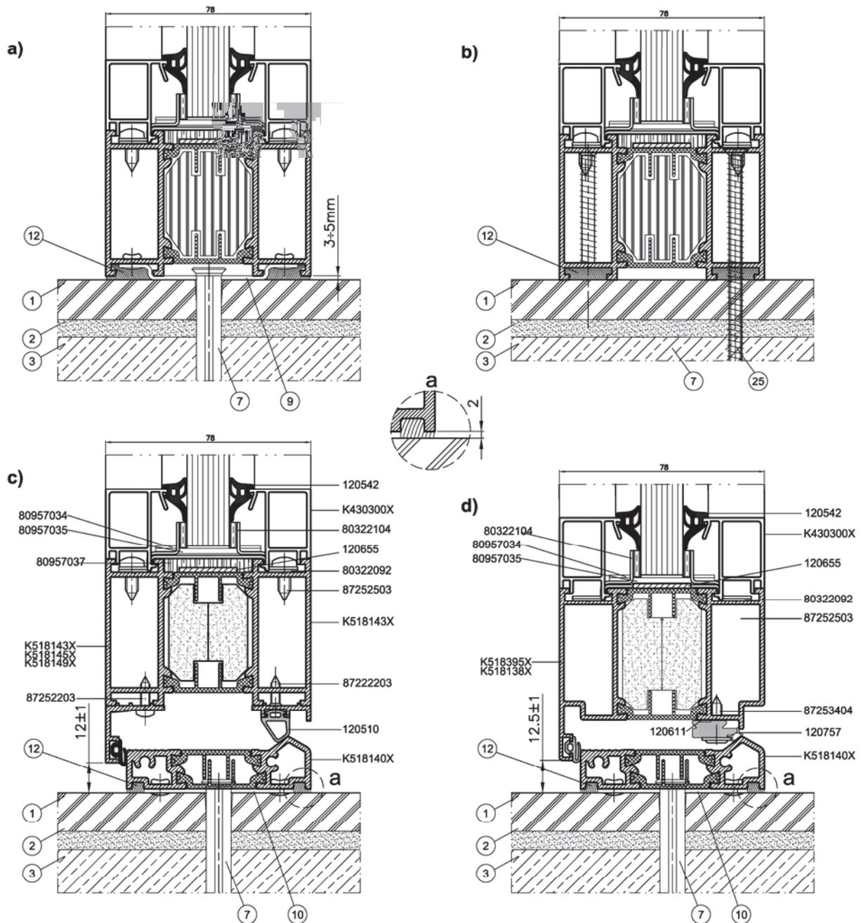
**Fig. 28 Clearances of base connection when installing:**
